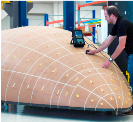
Ultrasonic NDI test on VEGA fairing
